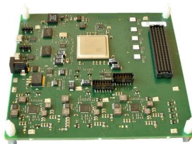
FPGA Printed Circuit Board – Front Side
